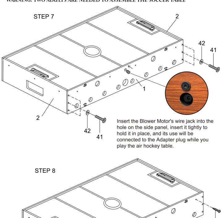
The Blower Motor jack into the hole on the side panel, which will be used to connect to the Adapter (#37).
