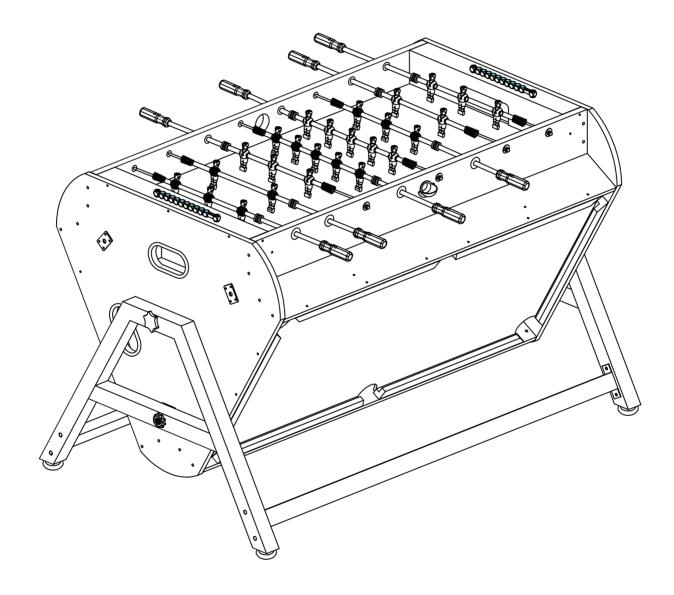
**NOTE:** Once table is completely assembled and placed in desired location, use level (not included) to adjust leg levelers so table is level in both directions.
