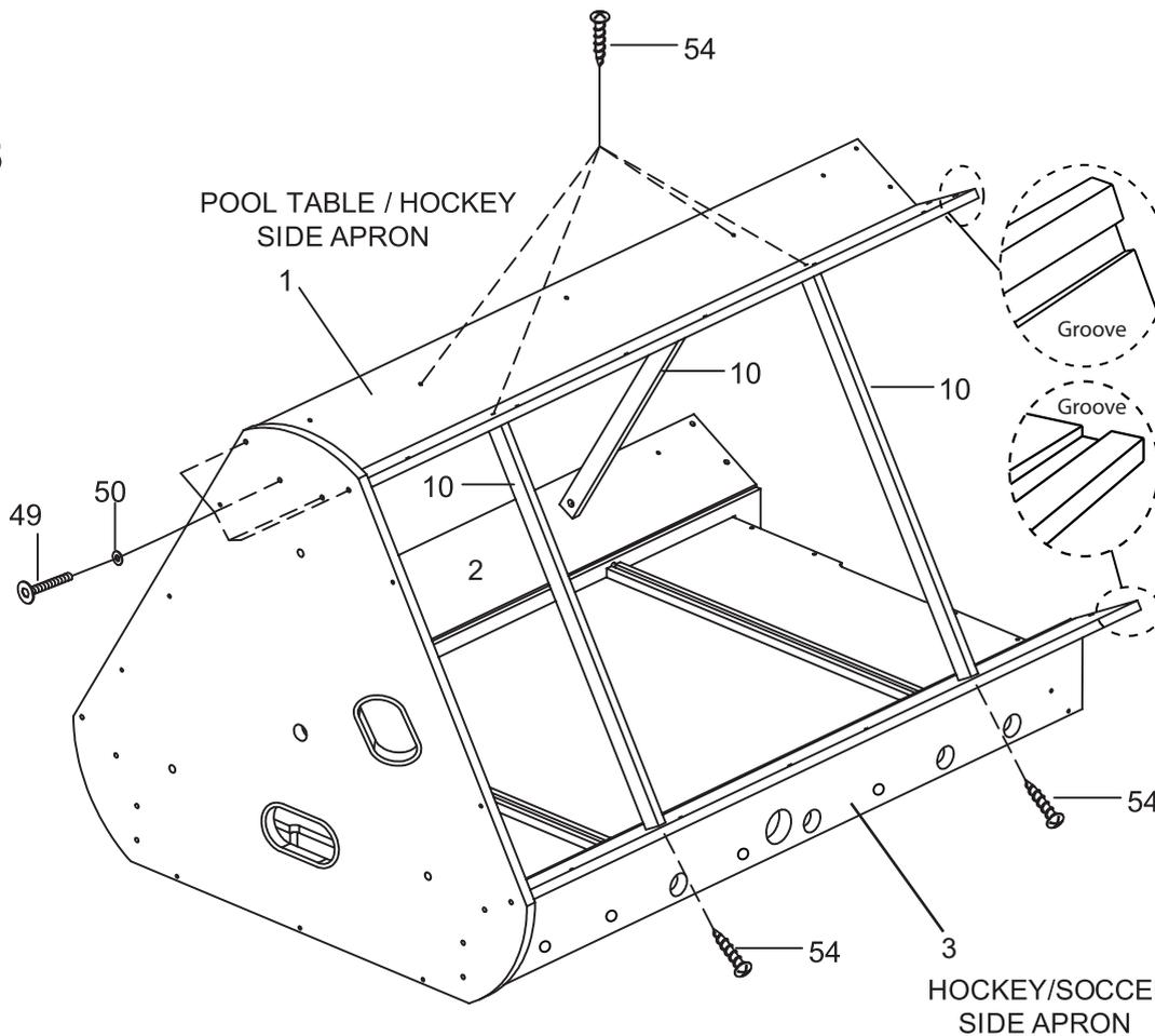
**Important Note:** There are grooves these positions of Pool Table/Hockey Side Apron (1) and Hockey/Soccer Side Apron (3), the grooves are for installing the Hockey Board (4) in the next step!
