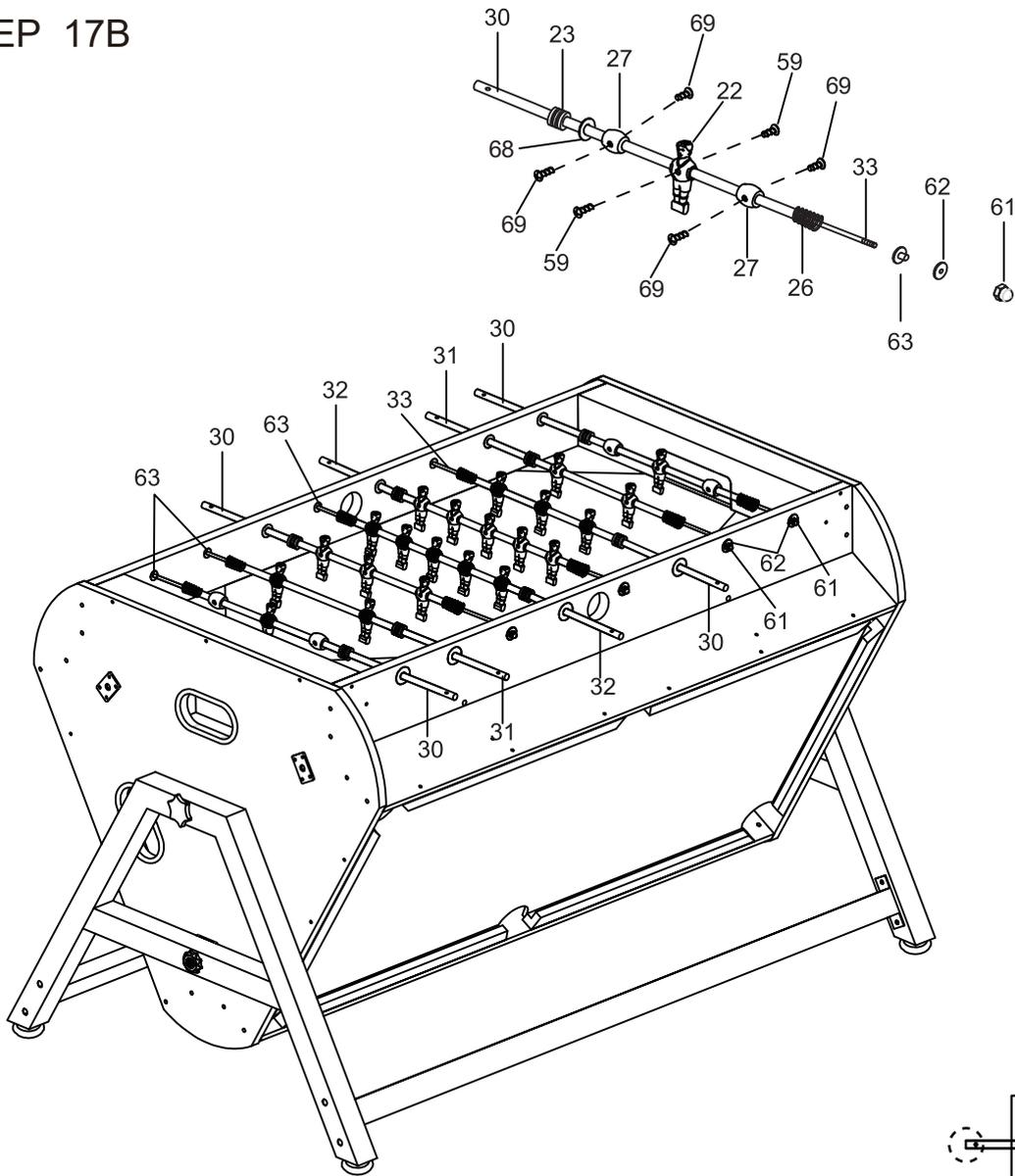
*Insert the rod end part way through one side panel, and then place the rest of the parts needed on each rod, in the order shown, before inserting through the other side panel.*
