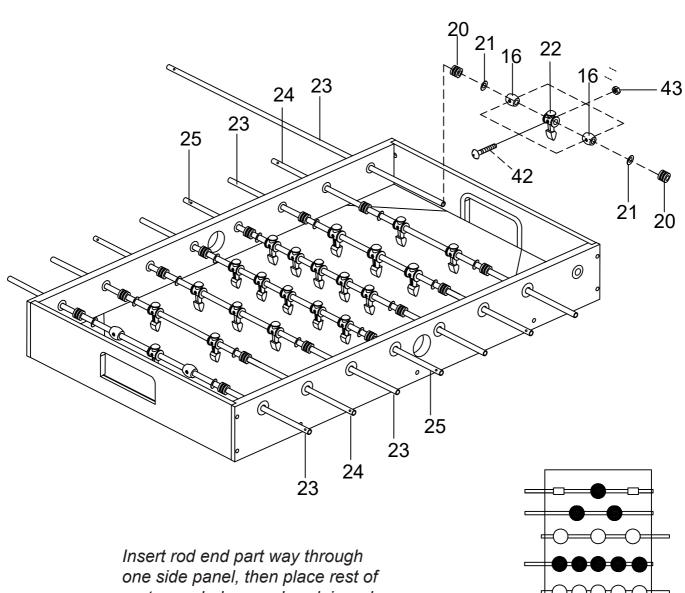
Insert rod end part way through one side panel, then place rest of parts needed on each rod, in order shown, before inserting through other side panel.
